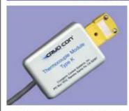
The Thermocouple module plugs into any of the standard input channels and is powered by the instrument. It provides amplification, cold-junction compensation and connection to copper. Thermocouple types can be selected using internal switches. Up to four modules can be connected to a single instrument.
