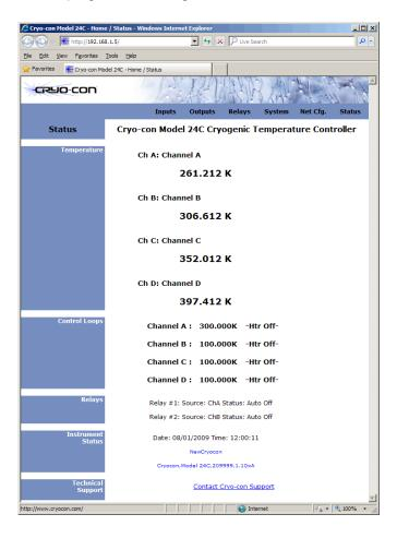
Using the Ethernet **HTTP** protocol, the instrument's **embedded web server** allows the instrument to be viewed and configured from any web browser.
